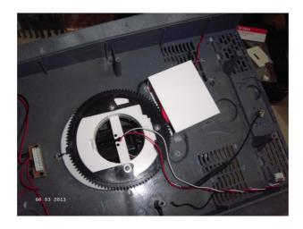
Glue the box with turret rotation unit to the underside of the hull.
