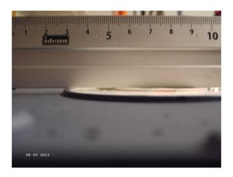
Move the ring with adapter from the underside into the turret ring. Check the gap. If there is a gap as in the above picture, proceed to the next step. If there is no gap then make adjustments with 1mm plates
