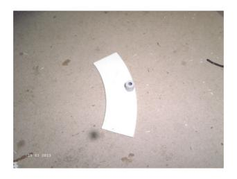
Glue the fixing point to the box plate
