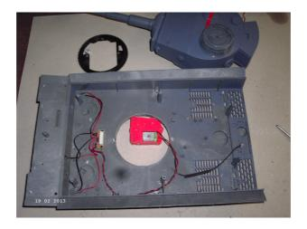
Disassemble the upper hull and remove the turret and turret rotation unit.
