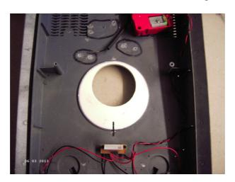
Position the adapter with the cutout slot to the centre mark.
